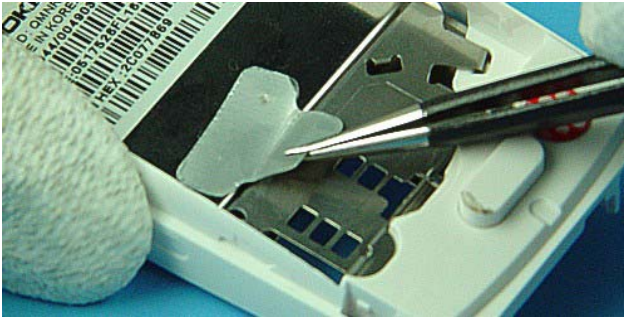
17) Remove the SIM Label with tweezers.
