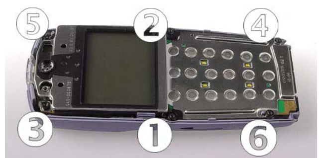
8) Unscrew the six Torx Plus® size 6 screws. For assembly, the reverse order and a torque driver with a torque of 20Ncm has to be used.
