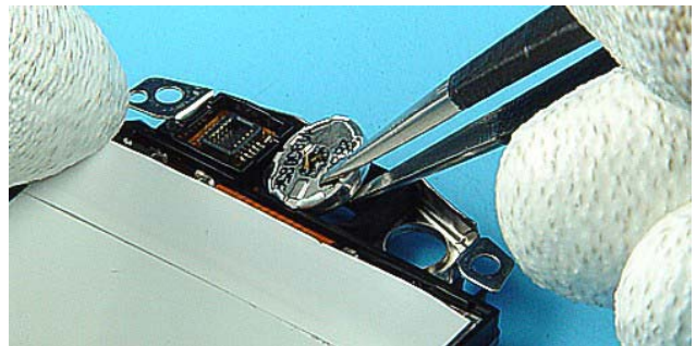
12) Remove the Earpiece with tweezers.
