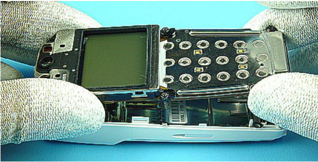
9) Remove the Engine Module include the LCD and Domesheet.
