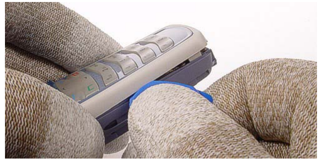
4) Use SRT-6 to remove the A-Cover .
