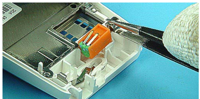
16) Remove the Vibra Motor with tweezers.
